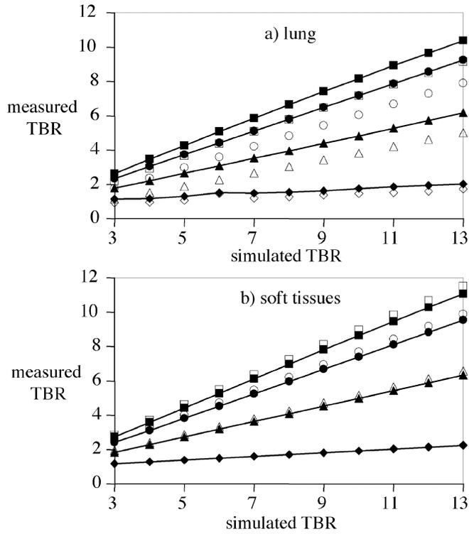
Fig. 7. Measured TBR with AC in (a) lung tumor; (b) soft-tissue tumor with  $FWHM_T = 8$  mm (empty symbol) and 4 mm (filled symbol) and  $FWHM_E = 4$  mm as a function of simulated TBR for lesion diameters of 4 cm (■), 2 cm (●), 1 cm (▲) and 0.5 cm (◆).
